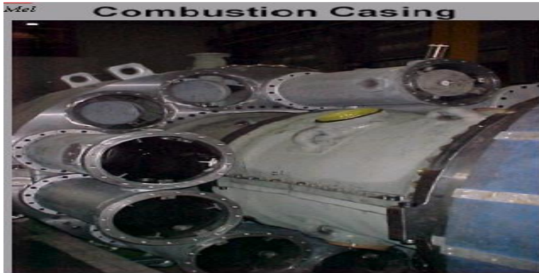
Figure .11 . Enveloppe de combustion
