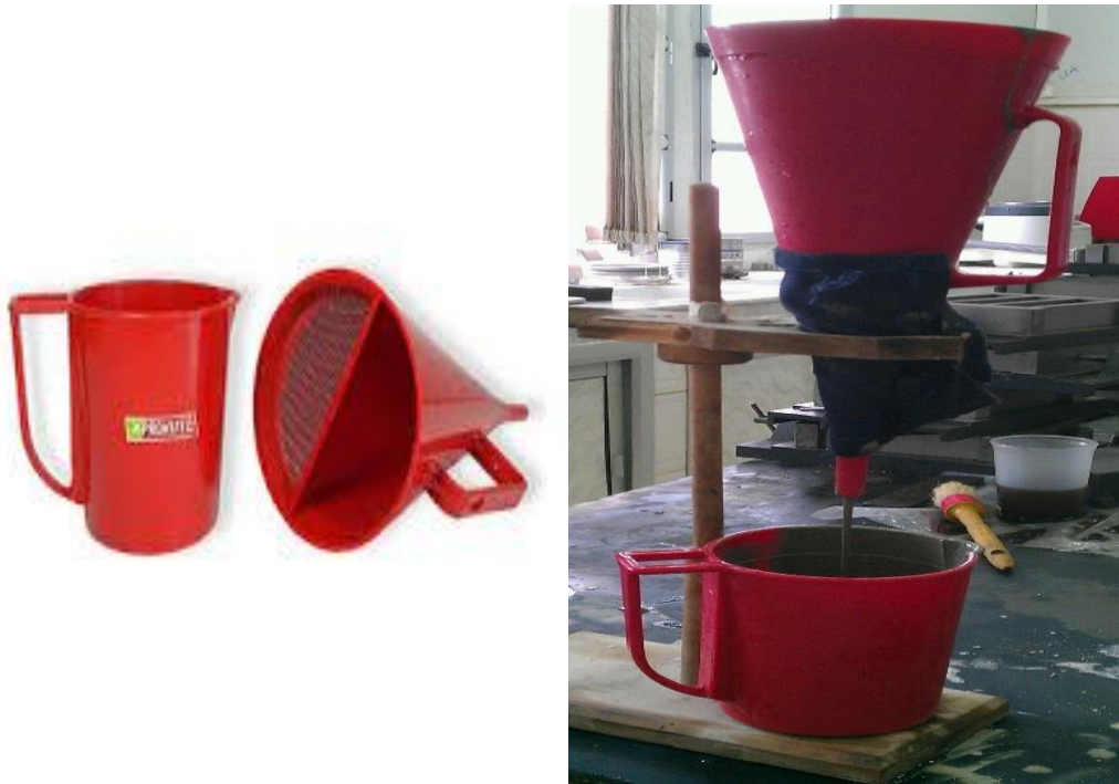
Figure II.3. Cône de Marsh.
