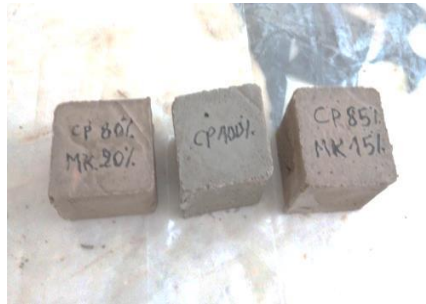
Fig.1 MK-metakaolin/Portland cement mortar specimens
