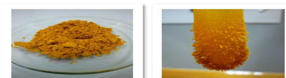
Figure 3(a)-(b). Purification of crude ferrocene via sublimation.
