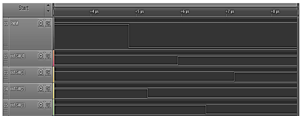
Figure 3-8: Signals at positive current falling edge
