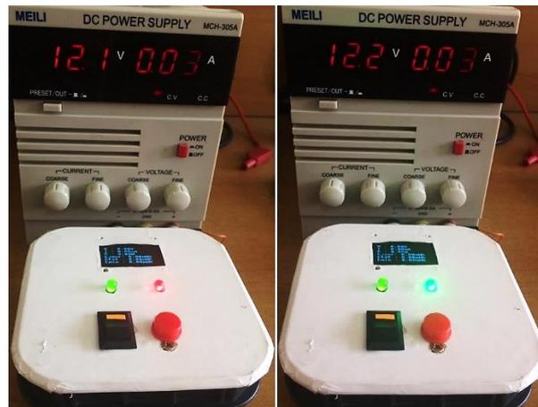
Si  $V_{\text{batterie}} < 12.2V$  | Si  $V_{\text{batterie}} \geq 12.2V$
