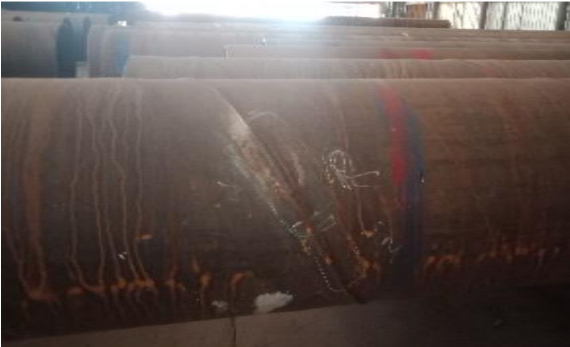
Figure 25 : the defects of weld bead
