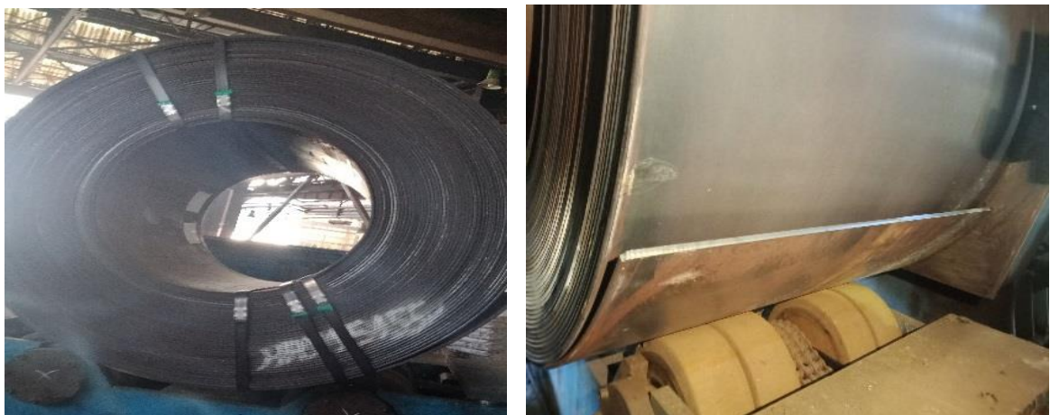
Figure 15:strip wound cold in spiral
