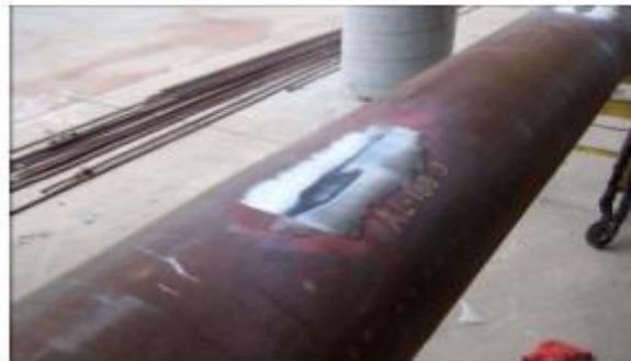
Figure 55: Scratch removed by grinding [7]
