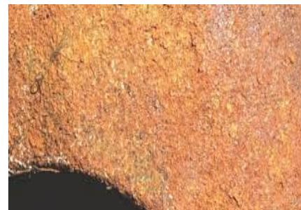
d. corrosion uniforme
