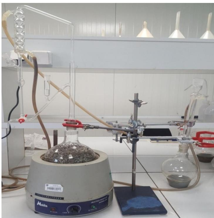
**Fig.11:** Dispositif de l'hydrodistillation (Clevenger) (CRD-SAIDAL, 2019)
