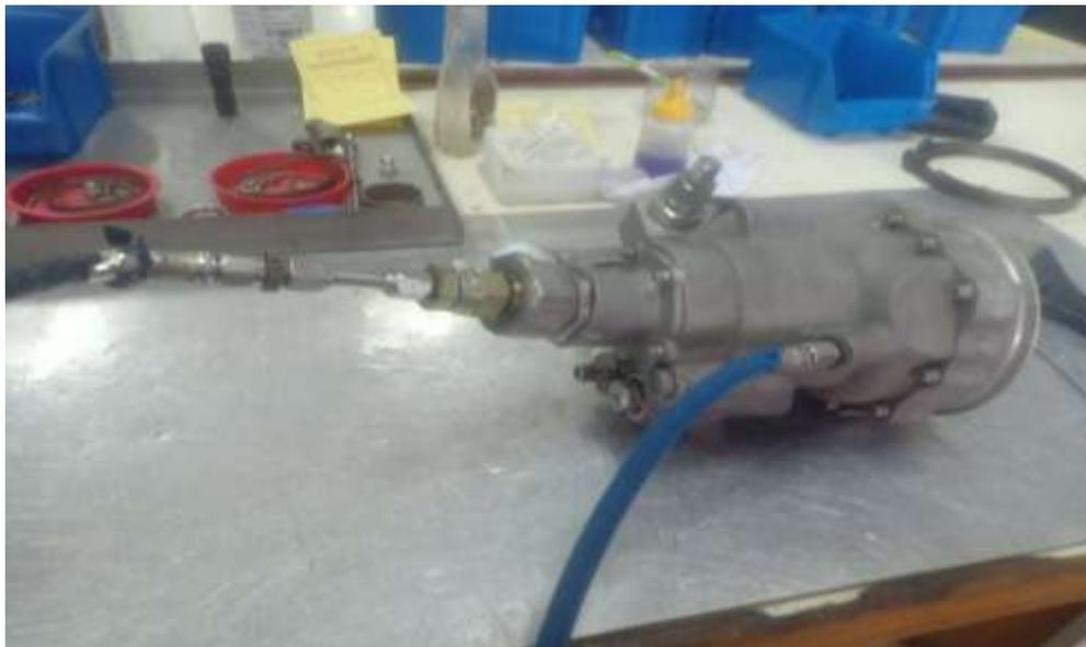
**Figure N°05: pompe hydraulique**
