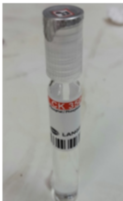
Figure A.12: cuve LCK350
