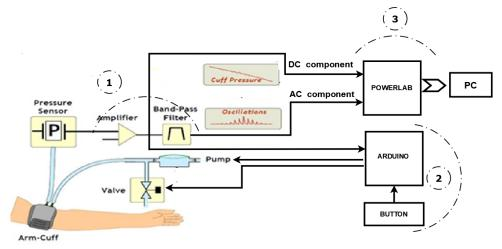
Figure 1: Diagram bloc of the oscillometric blood presure measurement
