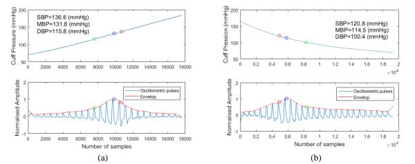
Figure 3: DC and AC signals and measurement of blood pressures found during cuff inflation and deflation. (a) during cuff inflation, (b) during cuff deflation
