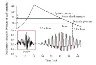
Figure 2 : SBP/DBP measurement technique in the Oscillometric methode.
