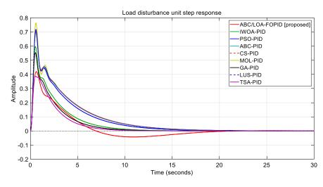
Figure 18. Disturbance rejection comparison for different techniques.
