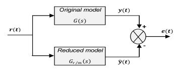
Figure 6. Error signal for model reduction.
