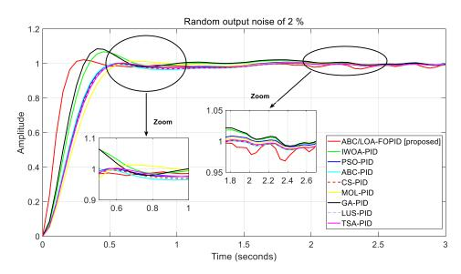
**Figure 16.** Controller's comparison with random output noise for 2% of the amplitude of the reference signal.
