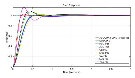
Figure 8. AVR terminal voltage comparison with existing techniques: IWOA-PID [21], PSO-PID [12], ABC-PID [15], CS-PID [26], MOL-PID [28], GA-PID [12], LUS-PID [31], and TSA [23].
