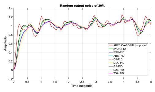
**Figure 17.** Controller's comparison with random output noise for 20% of the amplitude of the reference signal.
