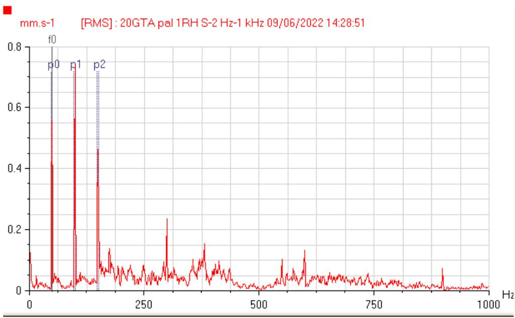
*Figure IV.7 Spectre de palier 1 Direction horizontale*
