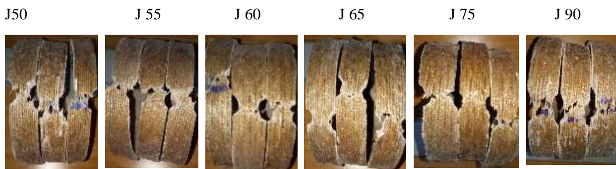
Figure IV 29 .Faciès de rupture Jute/Epoxy
