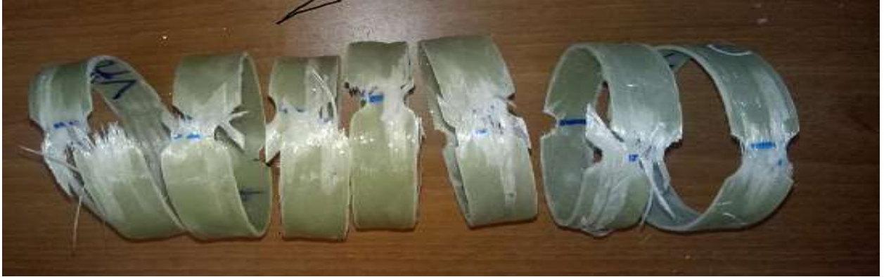
Figure IV 30. Faciès de rupture Verre/Epoxy
