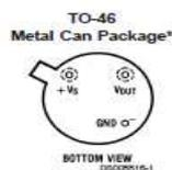
\*Case is connected to negative pin (GND)
