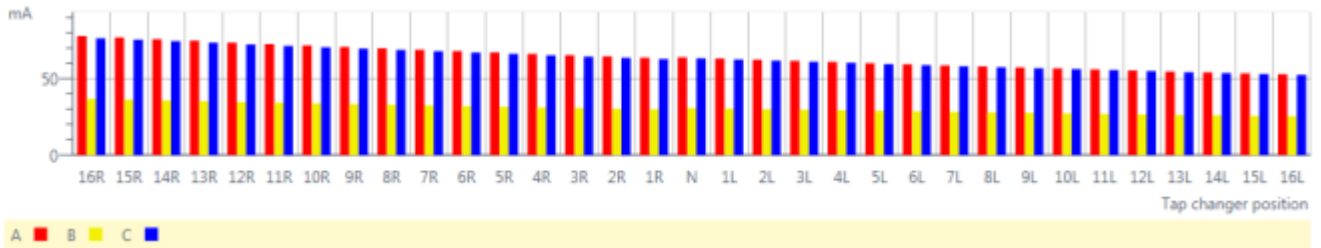
Figure A.7: Typical Tap-Changer Pattern when Resistive LTC is Located on Primary Side
