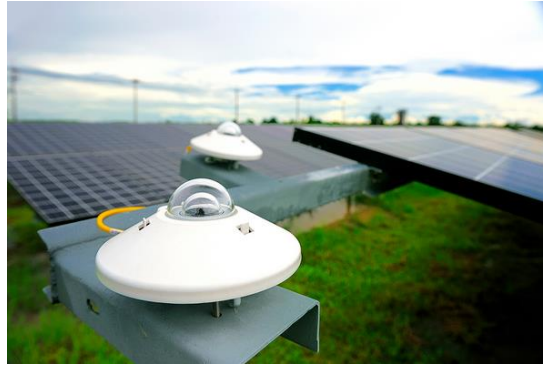
Figure 3.4: Kipp & Zonen CMP 22 pyranometer LI-COR pyranometer.
