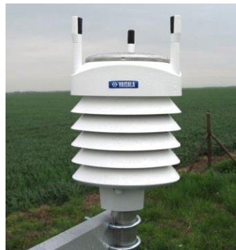
Figure 3.3: Vaisala Weather Transmitter WXT520 sensor [40].
