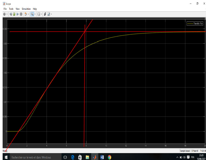
Fig II.28 Process response to the unit step with the tangential lines drawn on it
