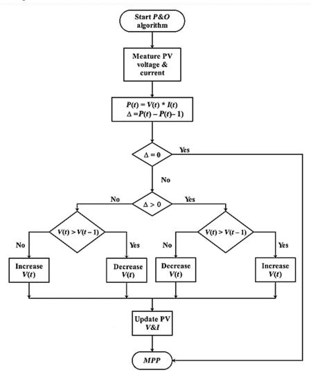
Figure 3. 7: Flowchart of P&O algorithm
