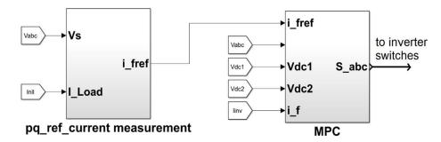
Figure 3. 10: Blocks Diagram of PQ Reference Current Measurement And MPC
