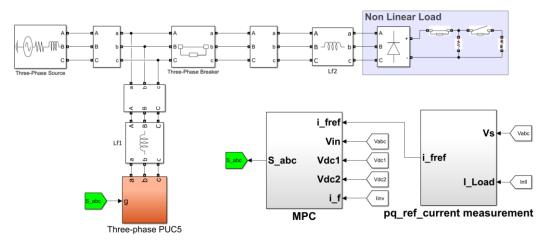
Figure B.1: Overall system diagram of PUC5 Three-phase inverter-based Solar-AF
