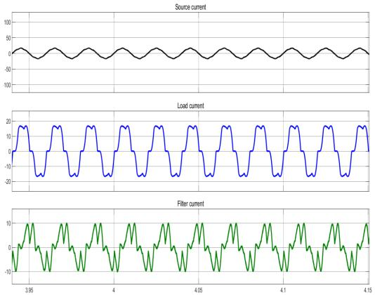
**Figure 4. 17**: Display of grid current, load current and filter current under zero irradiance.
