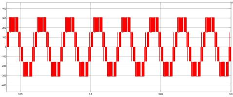
Figure 4. 30: demonstration of a one phase output voltage of PUC5 inverter
