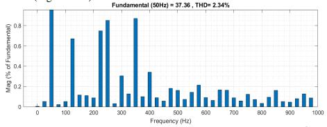
Figure 4. 12: FFT analysis tool for the source current under 500W/m<sup>2</sup>
