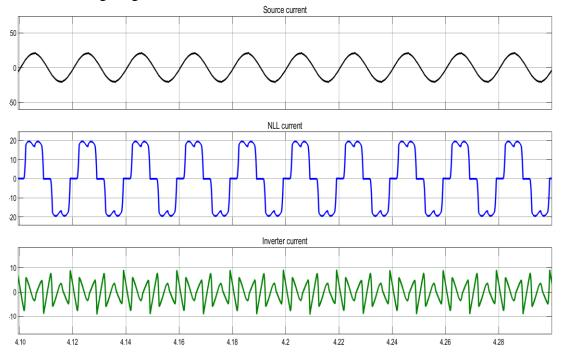
Figure 4. 33: Demonstration grid current, load current and filter current under  $0 \text{ W/m}^2$  (PUC5 inverter)
