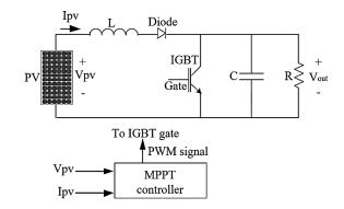
Figure 2. 12: DC-DC boost converter with MPPT
