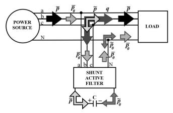
**Figure 3. 2:** Compensation of power components  $\tilde{p}$ , q,  $\tilde{p}0$  and  $\overline{p}0$  in a-b-c coordinates
