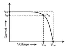
Figure 2. 7: V-I characteristics of PV array
