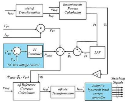
Figure 3. 3: p-q modified power injection
