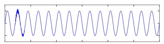
Figure 1. 7 Voltage waveform during noise
