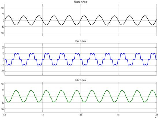
Figure 4. 11: Display of grid current, load current and filter current under 500W/m<sup>2</sup>
