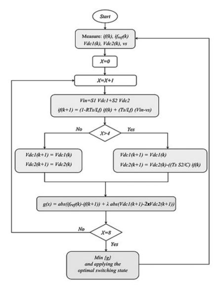
Figure 3. 9: Flowchart of the proposed MPC
