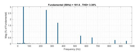
Figure 4. 18: FFT analysis tool for the source current under  $0 \text{ W/m}^2$
