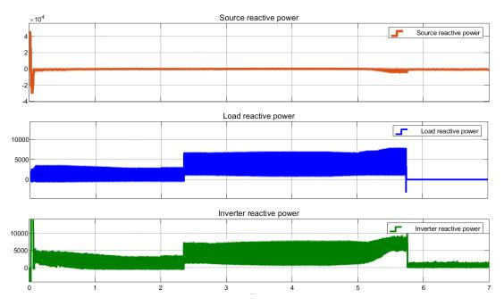
**Figure 4. 8**: A) Source, load and inverter reactive power in all the simulation using classical inverter
