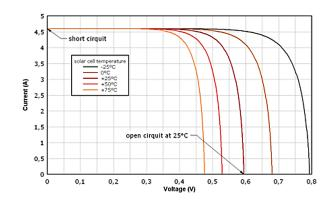
Figure 2. 9: I-V Characteristics for different temperature values
