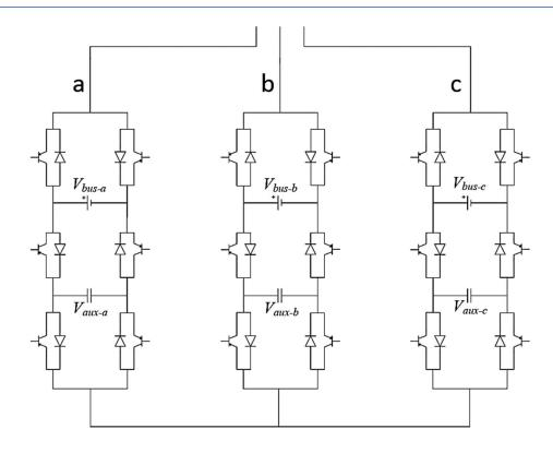
Figure 3. 8: PUC5 Three Phase Inverter Topology 3.5.1 Model Predictive Control (MPC)
