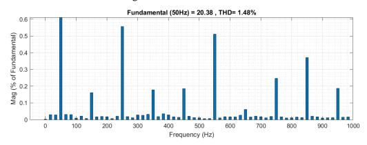
**Figure 4. 34**: FFT analysis tool for the source current of the system under 0 W/m<sup>2</sup> (PUC5 inverter)
