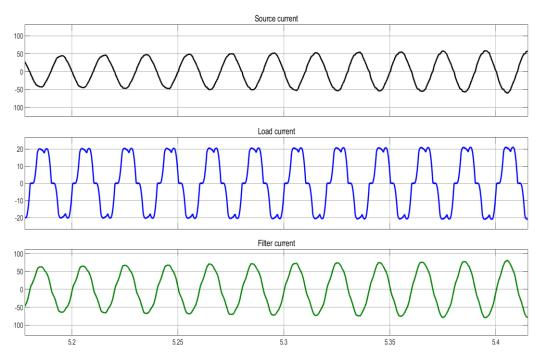
Figure 4. 19: Display of grid current, load current and filter current during increasing irradiance condition.
