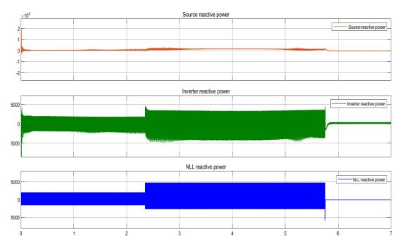
**Figure 4. 27:** Source, nonlinear load and inverter reactive power in all the simulation using PUC5 inverter
