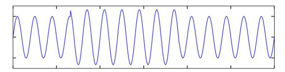
Figure 1. 5 Voltage waveform during swell
