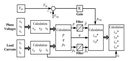
Figure 3. 1: Calculations for the constant instantaneous supply power control strategy
