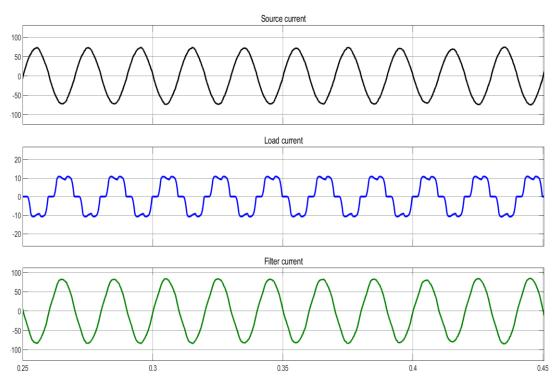
Figure 4. 9: Display of grid current, load current and filter current under 1000W/m<sup>2</sup>
