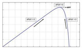
Figure 3. 6: Workflow of P&O algorithm in P-V characteristics
