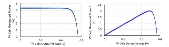
Figure 2. 4: Current vs voltage (I-V) characteristics of PV cell and power vs voltage (P-V) characteristics of PV cell.
