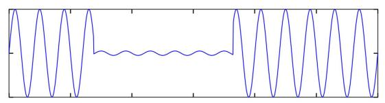
Figure 1. 3 Voltage waveform during an interruption
