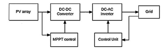
Figure 1. 1 Grid connected PV system
