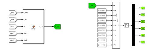
Figure B. 2: MPC scheme per phase
