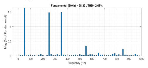
**Figure 4. 16**: FFT analysis tool for the source current under 600W/m<sup>2</sup> with extra load demand
