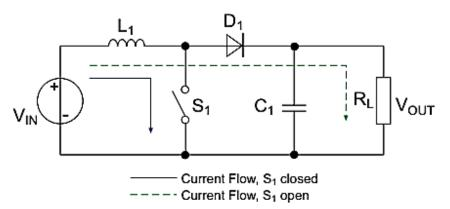
Figure 2. 11: Current flow across boost converter according to the switching states
