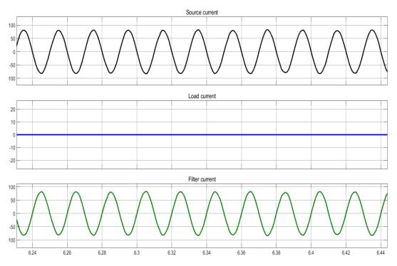
Figure 4. 21: Display of grid current, load current and filter current under no load condition.
