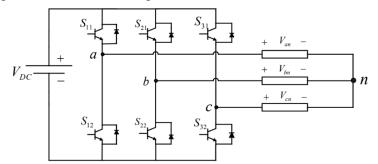
Figure 2. 13: Two-level three-phase inverter
