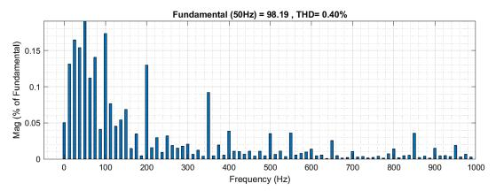
Figure 4. 32: FFT analysis tool for the source current of the system under  $1000 \text{ W/m}^2(\text{PUC5 inverter})$
