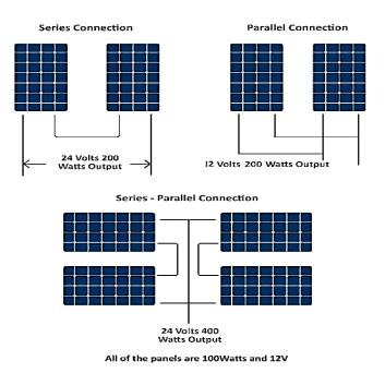
in an array can be electrically connected in either a series, a parallel, or a mixture of the two.
