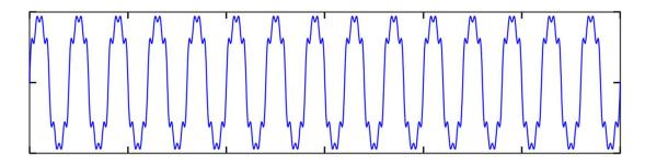
Figure 1. 6 Voltage waveform during harmonics
