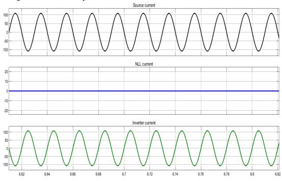
Figure 4. 36: Demonstration grid current, load current and filter current without load
