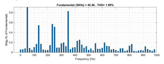
**Figure 4. 14**: FFT analysis tool for the source current under 600W/m<sup>2</sup>
