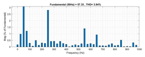
**Figure 4. 20**: FFT analysis tool for the source current System under 1000 W/m<sup>2</sup> with extra load demand
