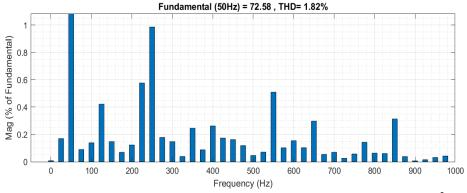
Figure 4. 10: FFT analysis tool for the source current under 1000W/m<sup>2</sup>
