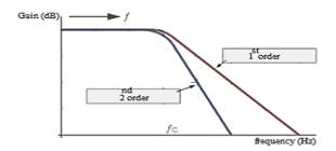
Figure 2. 16: Frequency response of 1<sup>st</sup> order and 2<sup>nd</sup> order low pass filter
