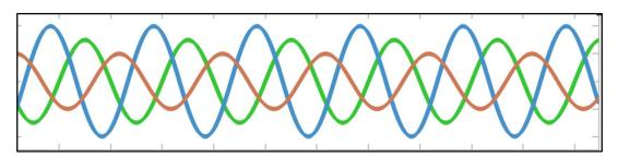
Figure 1.9 Voltage waveform during voltage unbalance.
