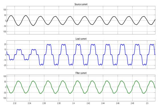
**Figure 4. 15**: Display of grid current, load current and filter current with additional load demand
