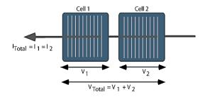
Figure 2. 5: Series connected PV cells
