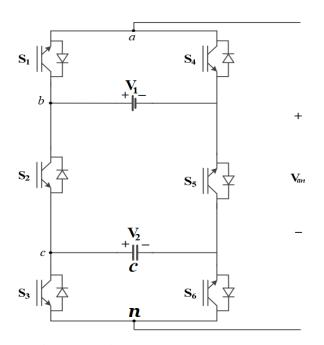
Figure 2. 14: Single-phase PUC Inverter
