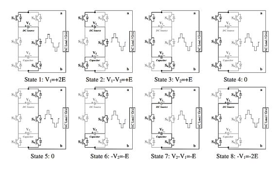
Figure 2. 14: PUC5 configuration, switching states and conducting paths
