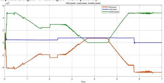
Figure 4. 7: Active power curves of source, load and inverter during the simulation time using classical inverter
