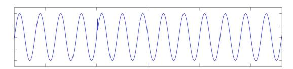
Figure 1. 4 Voltage waveform during spike
