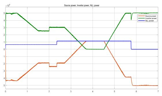
Figure 4. 26: Active power curves of source, load and inverter during the simulation time using PUC5 inverter
