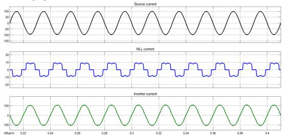
Figure 4. 31: demonstration of grid current, load current and filter current under  $1000W/m^2$  (PUC5 inverter)
