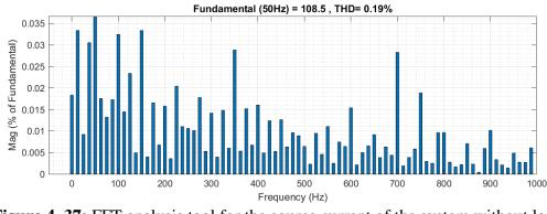
Figure 4. 37: FFT analysis tool for the source current of the system without load (PUC5 inverter)
