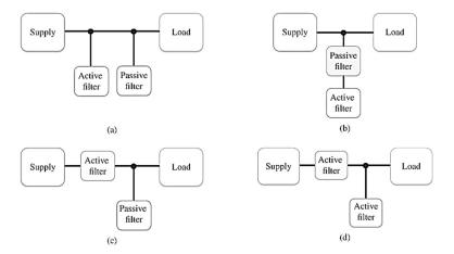
FIGURE 1. 13 Hybrid connections of active and passive filters.
