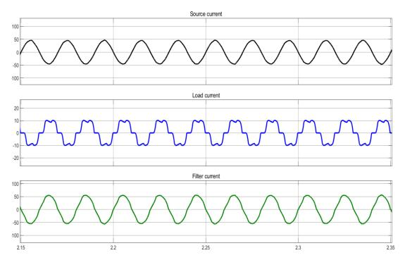
Figure 4. 13: Display of grid current, load current and filter current under 600W/m<sup>2</sup>
