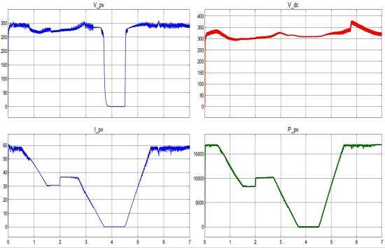
Figure 4. 24: Demonstration PV Output Voltage, Current, Power and The DC Link of phase A for All the Simulation using PUC5.
