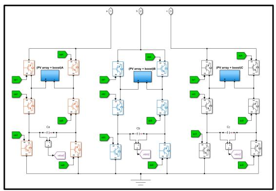
Figure 4. 23: the simulated system of the three phase PUC5 inverter-based Solar-AF
