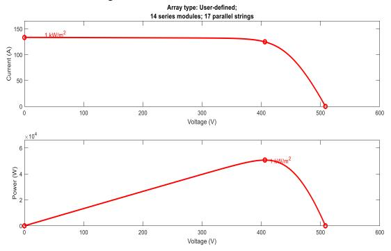
Figure 4. 2: The I-V and P-V characteristics of the used PV module (under STC)
