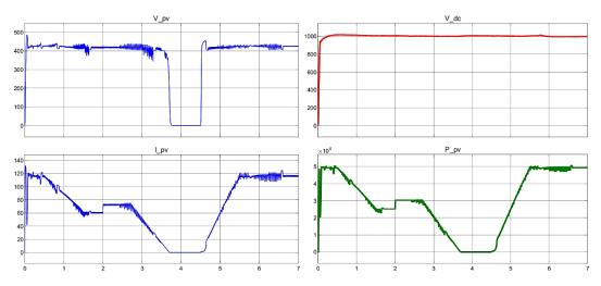
Figure 4. 6: Demonstration PV Output Voltage, Current, Power and The DC Link for All the Simulation using the classical inverter.
