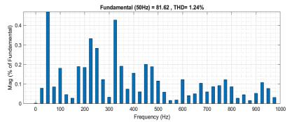
Figure 4. 22: FFT analysis tool for the source current of the system without load
