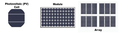
Figure 2. 1: photovoltaic cell, module and array
