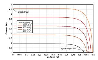
Figure 2. 8: I-V characteristics for different irradiation values
