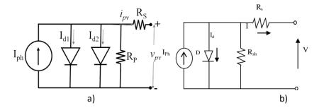
Figure 2. 3: a) Double and b) single diode models equivalent circuits
