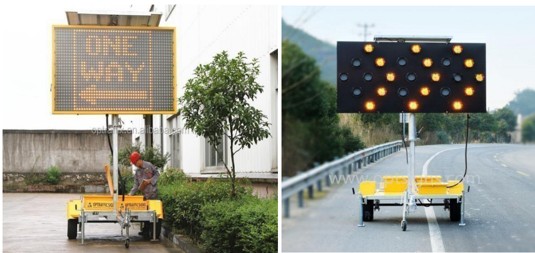
Figure I.3: The use of solar energy in mobile VMS [15].
