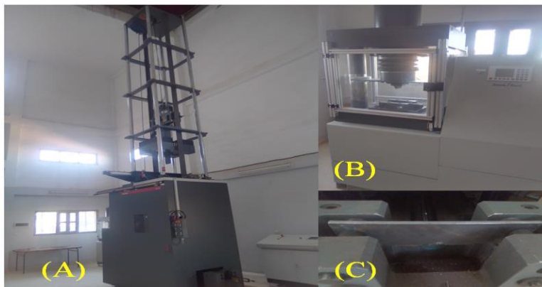
Figure 5. 3 Specimen used for DWTT and the impact machine for steel X70
