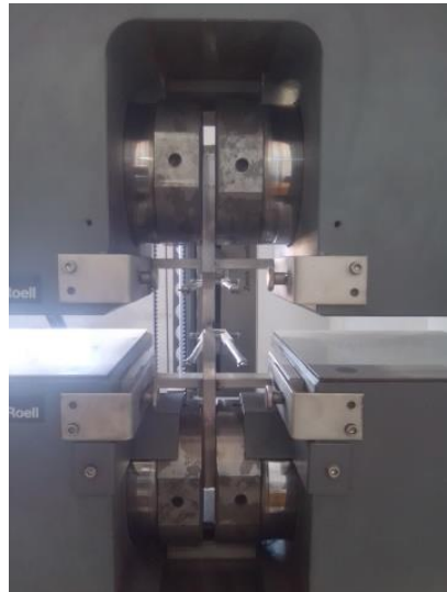
Figure 4. 5 Test specimen with a tensile extensometer in the tensile testing machine.
