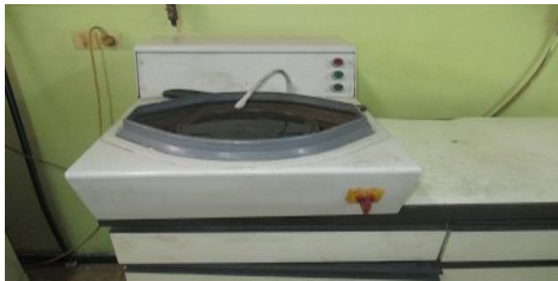
Figure 3. 10 Mechanical polishing with abrasive papers.
