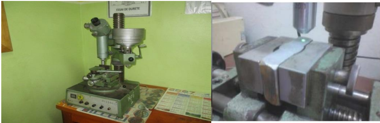
Figure 3. 12 Microhardness tester used for microhardness measurements (Vickers type).
