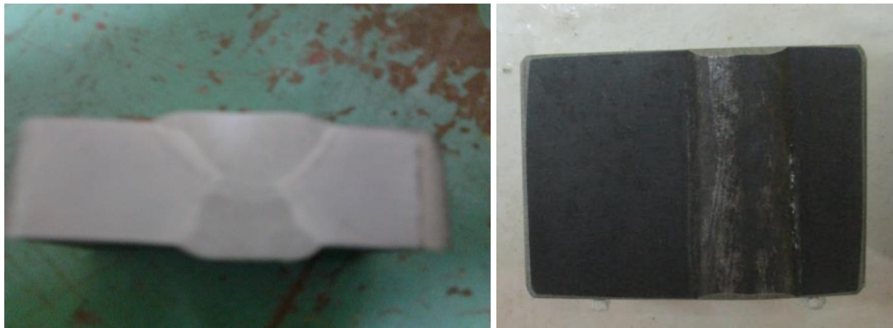
Figure 3. 11 Specimen for the microhardness test.
