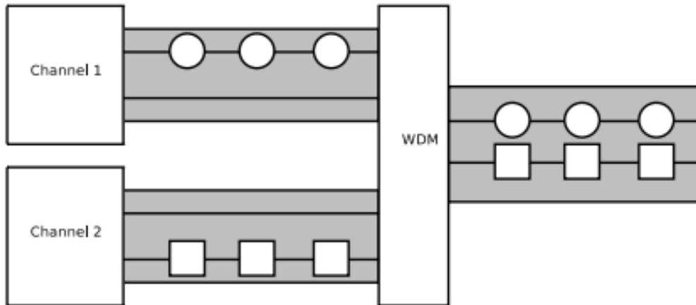
Figure 1.9: Simple schematic of a WDM system for  $N = 2$
