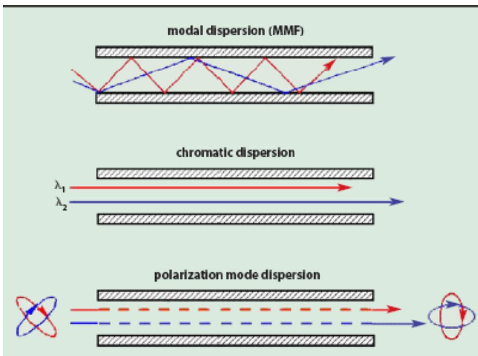
Figure 2.2: The three types of optical dispersion
