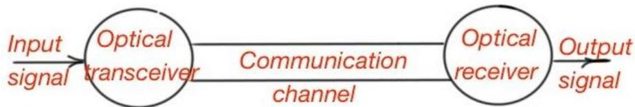
Figure 1.1 : basic configuration of optical fiber communication
