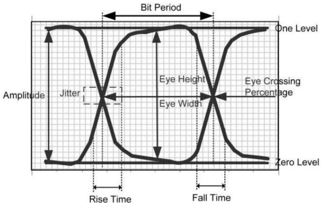
**Figure 1 :** Eye-Diagram Measurements .
