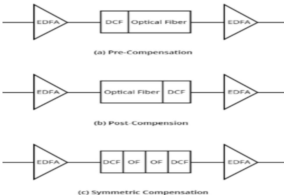
Figure 3.2: transmission line model: a-pre-compensation, b-post-compensation, c- symmetric compensation
