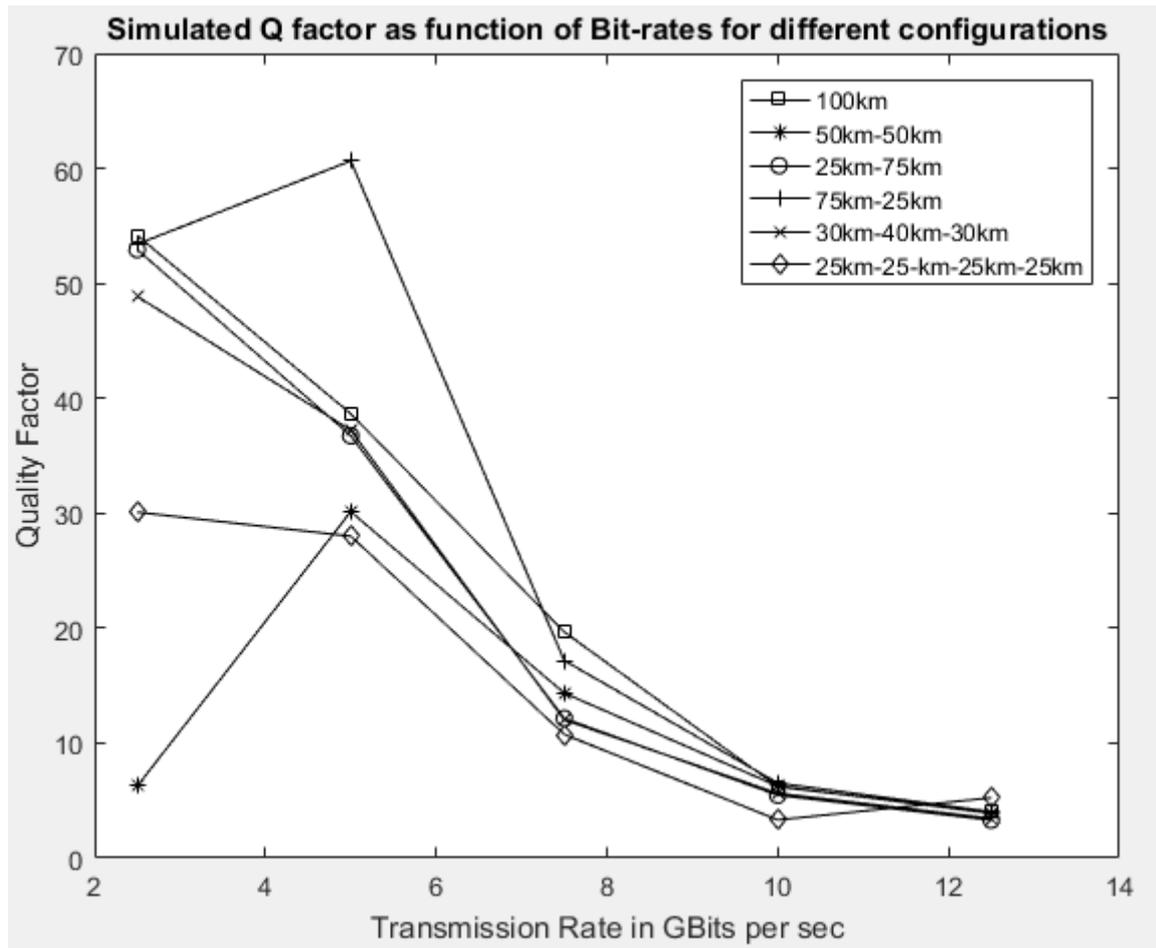
Figure 3.13 : Simulated Q factor as function f Bit-rates for different configurations
