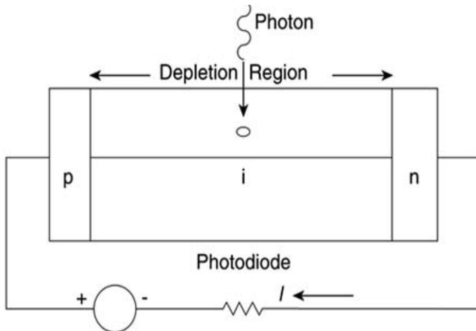
Figure 1.6: PIN photodiode
