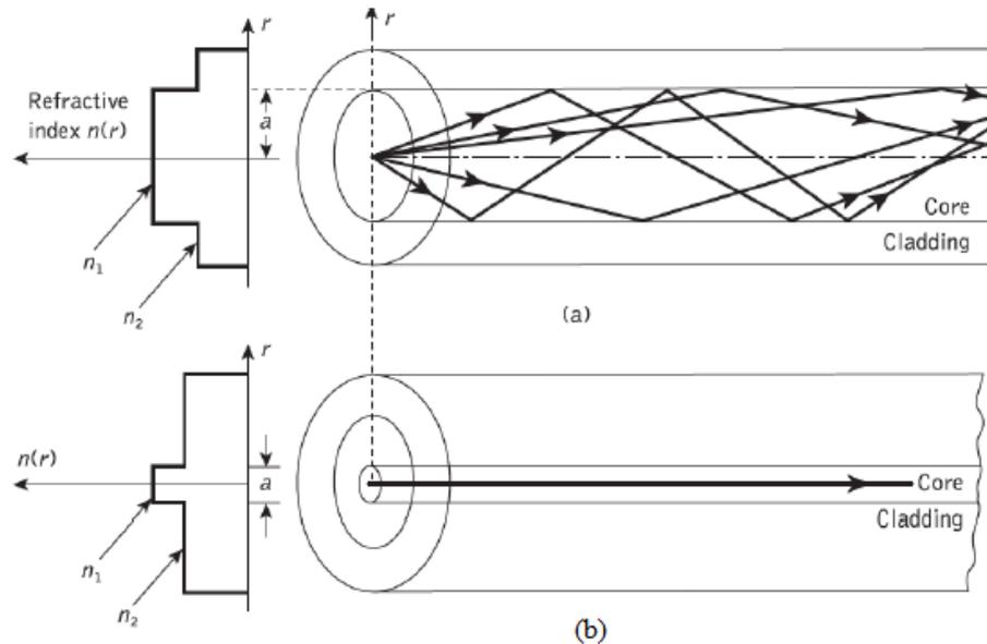
Figure 1.5: a) Multimode fiber b) Single mode fiber.
