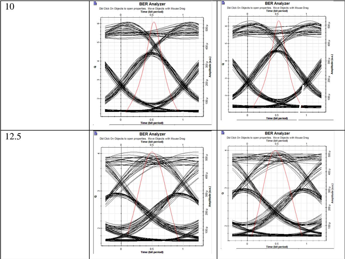
From tables 3.7, 3.8 and 3.9, the 75-25 km configuration gives higher Q factor and wider eye diagrams in all channels for the 5Gbps and 10Gbps bit rates, and in ch-1 and ch-8 for 2.5Gbps. Hence for the others bit rates the 100 km configuration results are better except in ch-16 for 12.5 Gbps.
