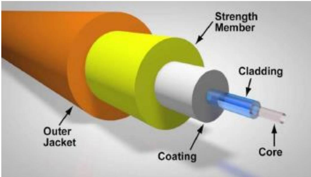
Figure 1.2 : structure of an optical fiber [3]
