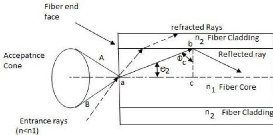
Figure 1.4 : signal propagation in optical fiber
