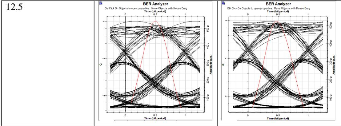
From tables 3.4, 3.5 and 3.6, in channel 1 and channel 8 the 75-25 km configuration gives better results for 2.5Gbps and 5Gbps we have got higher Q factor and wider eye diagrams but as a higher data rate is transferred, the 100 km configuration Seems more convenient for the same channels. In the other side, the results obtained in channel 5, for 2.5 Gbps and 5 Gbps the 100 km configuration are slightly better and vice versa for the other bit rates.
