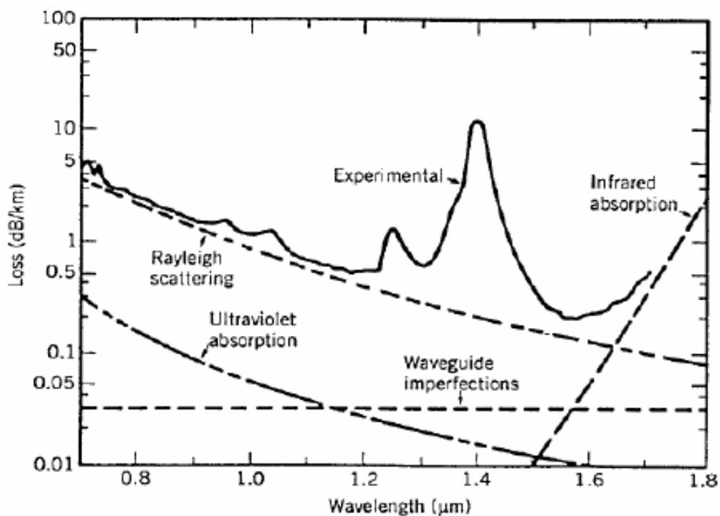
Figure 1.8: Optical fiber attenuation curve
