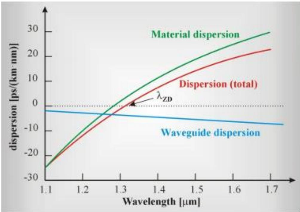
Figure 2.3: Total dispersion, material dispersion and the waveguide dispersion in a typical single mode fiber.
