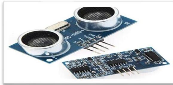
**Figure 1.10. HC-SR04 Ultrasonic sensor**
