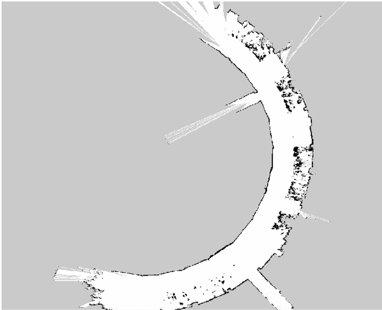
**Figure 4.2. map of the CDTA hallway using HECTOR SLAM**
