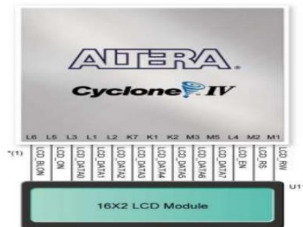
Figure 3-15: Connections between the LCD module and Cyclone IV E FPGA [20].
