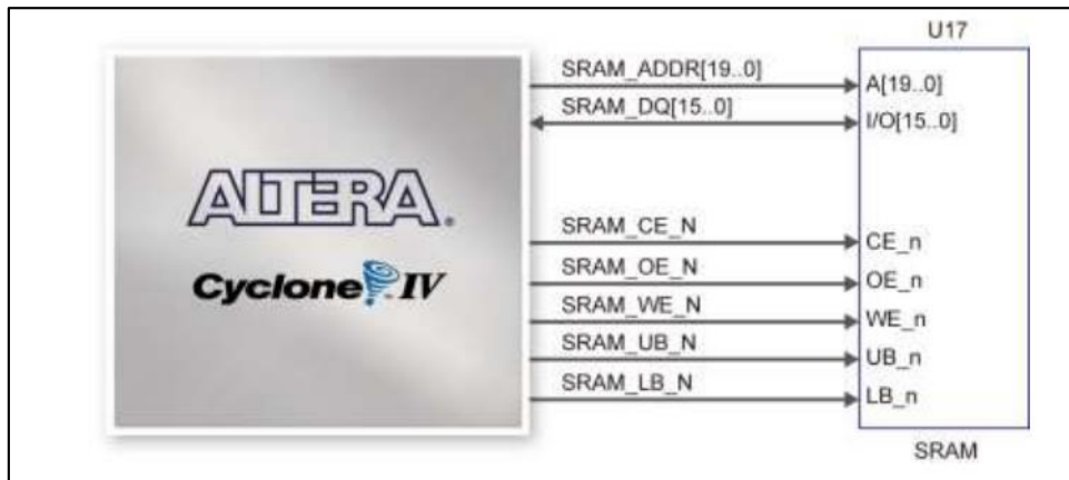
Figure 3-13: Connections between FPGA and SRAM [20].
