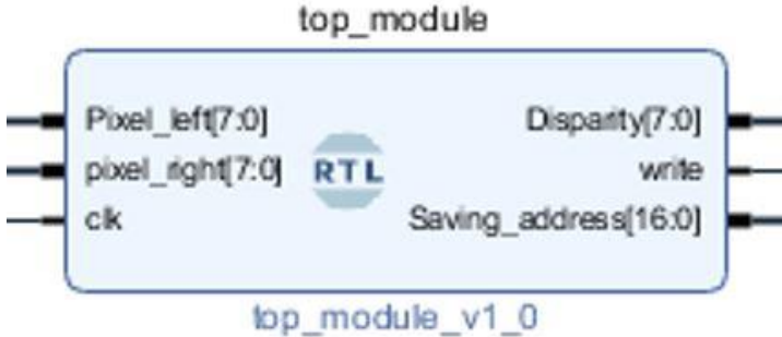
Figure III. 3: Matching module as a block.
