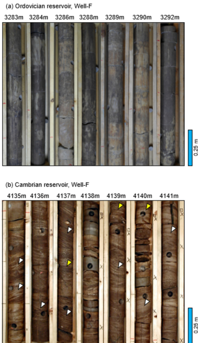
Fig. 5. Core photographs of the (a) Ordovician reservoir (3283–3292 m interval) and (b) Cambrian reservoir (4135–4141 m interval) in the Well-F. The Ordovician Formation consists of dark grey sandstones, devoid of any primary sedimentary structure. The Cambrian Formation consists of brownish grey sandstones exhibiting through cross stratifications (marked by white arrows) with minor planar horizontal laminations (marked by yellow arrows). The horizontal fractures seen in the core photographs were created due to the coring technique. The length of each core is 1 m (vertical scale is provided) and the core diameter is about 6 inches (15.24 cm).
