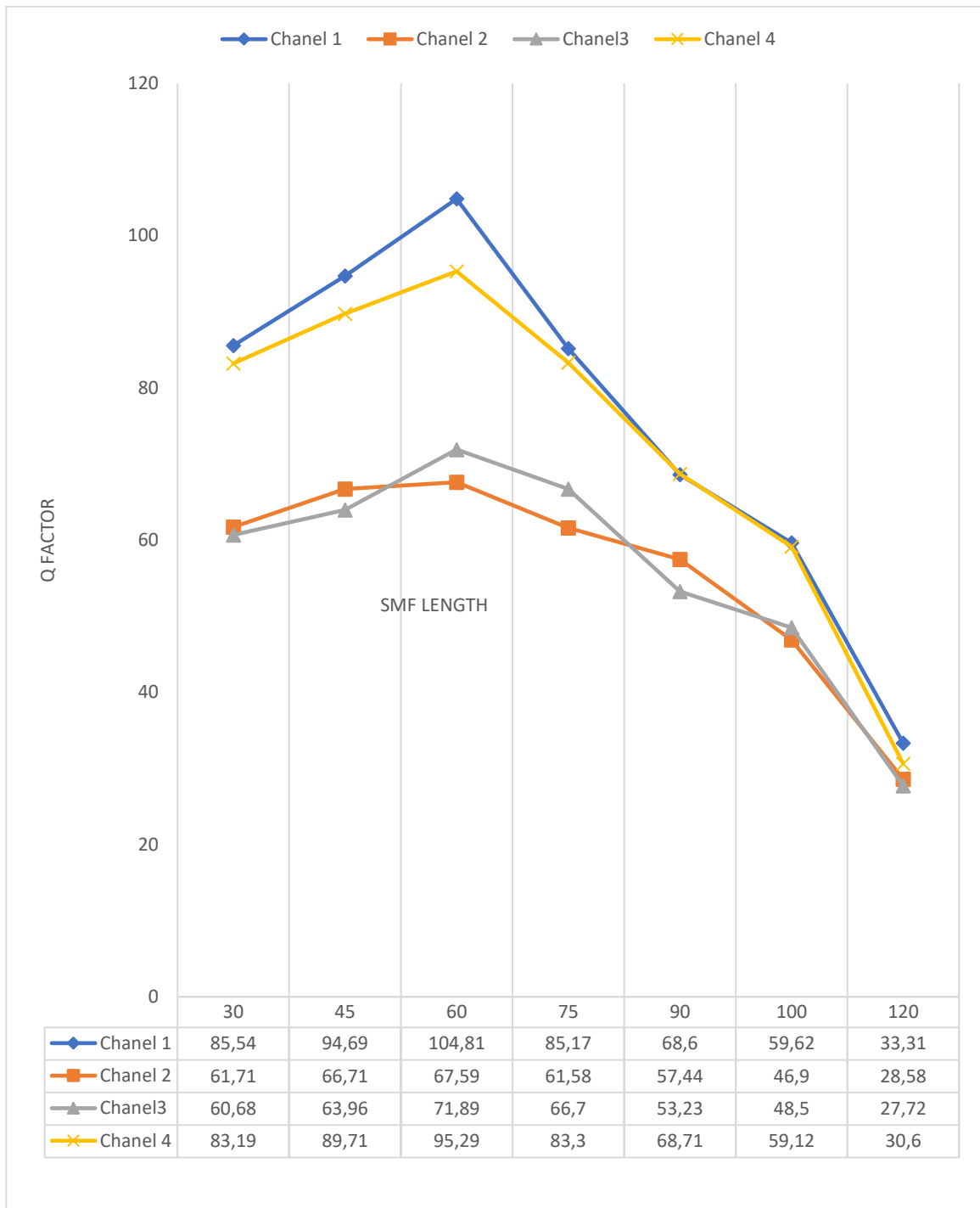
Figure 3.16: SMF length versus Q factor at 2.5 Gbps bite rates for 4-Channel WDM system using Pre-compensation.
