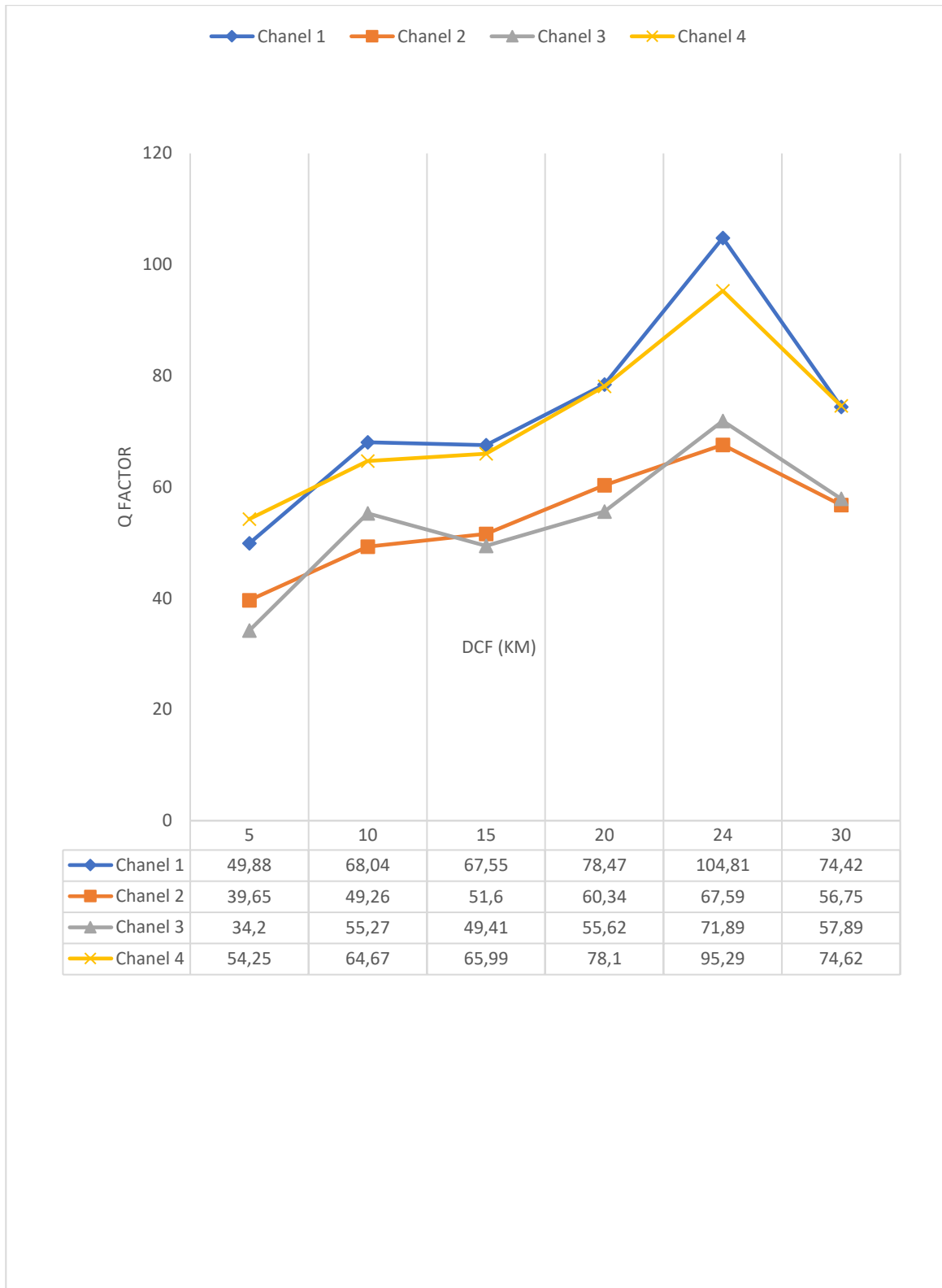
Figure 3.17: DCF length versus Q factor at 2.5 Gbps bit, 8 dBm power, 60km SMF length for 4-Channel WDM system using Pre-compensation.
