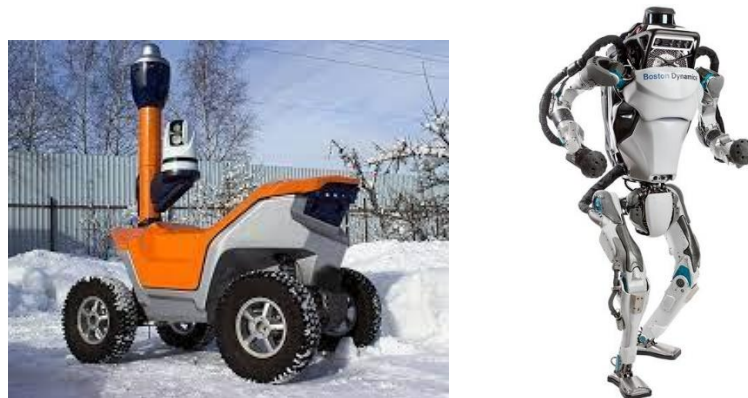
Figure1.2: (a). S5.2 outdoor security and inspection robot [21], (b). Atlas humanoid robot [20]
