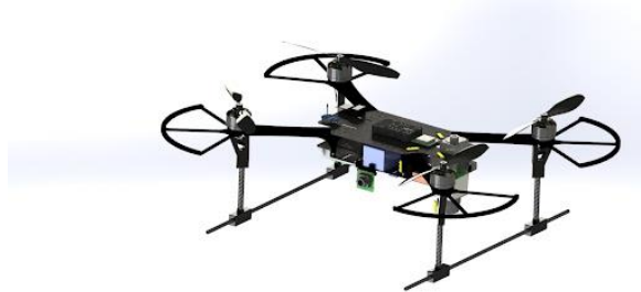
Figure1.3: ARSI, aerial robot for sewer inspection[22]
