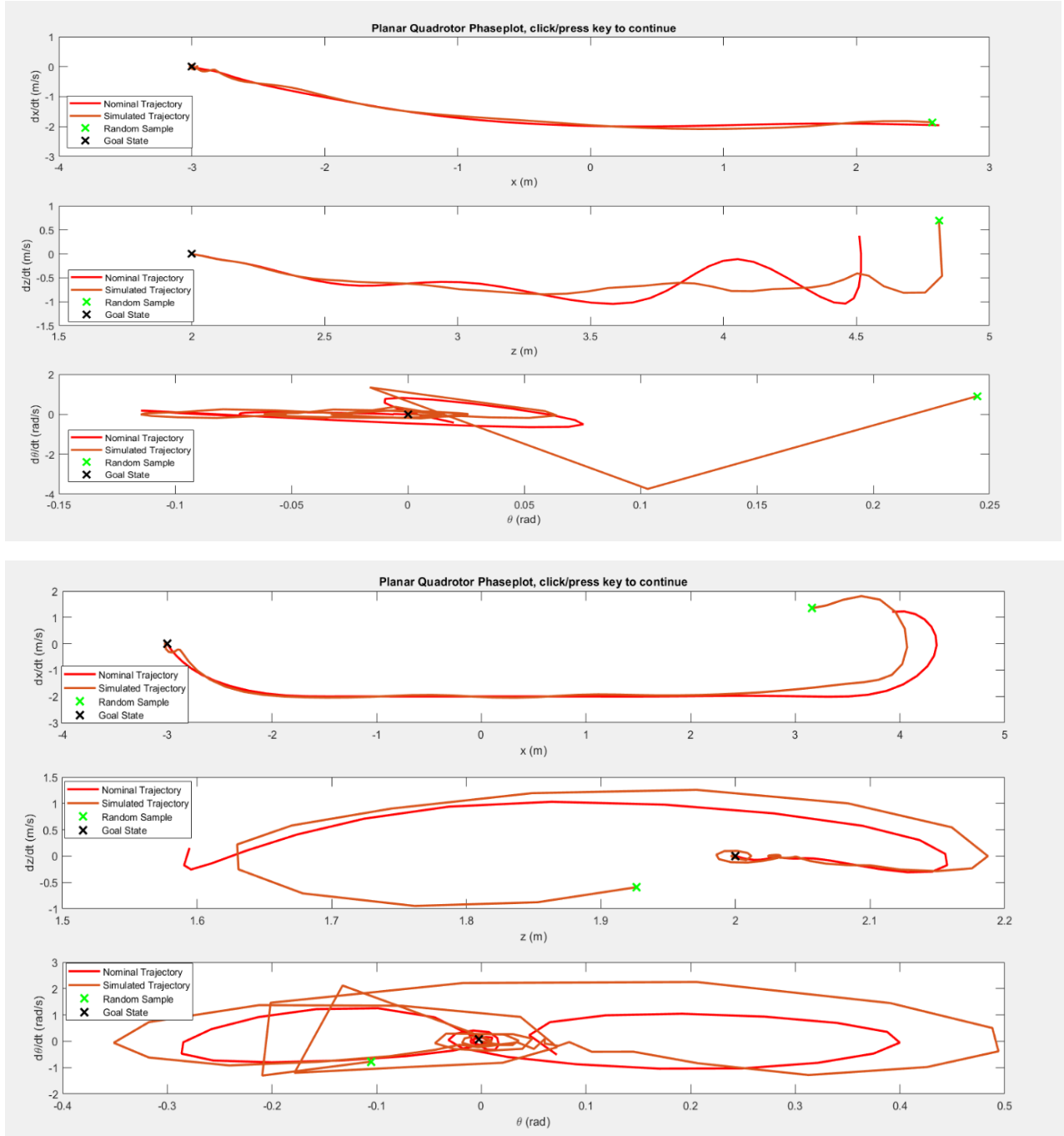
Figure 3-11: Phase plots of a two successful simulations. The red trajectory represents the nominal one whereas the brown trajectory represents the simulated one. The Green cross represents the initial state and the black cross represents the Goal state.
