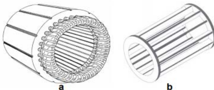
Figure 1.1 (a) A typical structure of stator core and (b) the rotor in squirrel-cage induction motor.
