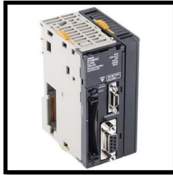
Figure 1.14: CPU module of an OMRON CJ1M PLC
