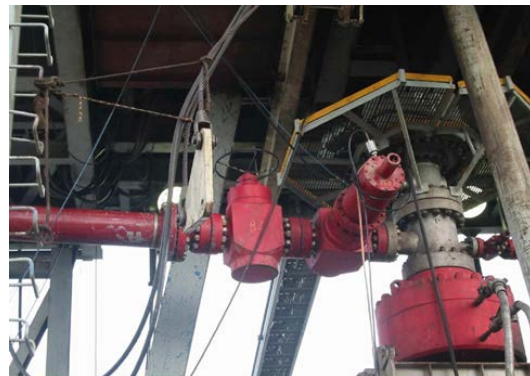
Figure II-23 - Flow line Principale
