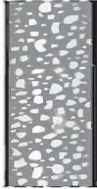
Figure II-4: Bubble Flow
