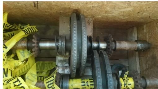
Figure II 1 rotor de turbine
