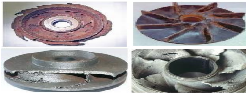
Figure I-11: Cavitation des pompes
