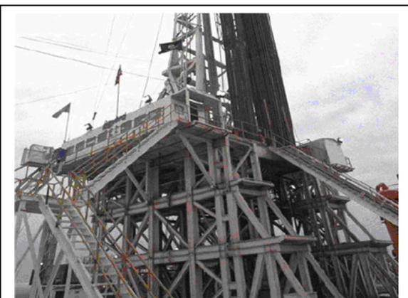
**Fig.II.4 : La substructure**
