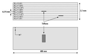
Fig 2. Typical location and size of delaminations
