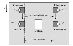
Fig 5. Schematic representation of line-scanning method
