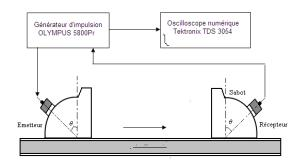
Fig 3: S<sub>0</sub> Lamb wave mode generation and detection.
