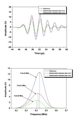
Fig 4: Waveform detected of two different delaminations
