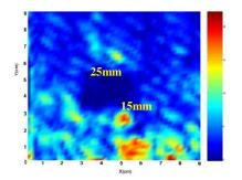
Fig 7.C-scan image of delamination
