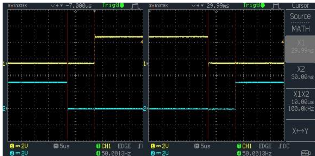
Figure 40. Zoomed-in view highlighting the 10us dead time in the control signals of the square wave inverter.
