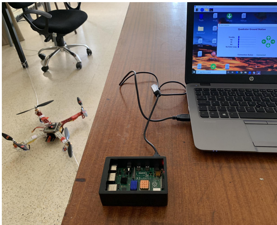
Figure 4.16: Quadrotor flight controller controlled wirelessly with Raspberry Pi GUI.
