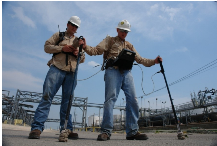
Figure 1.7: Direct Current Voltage Gradient (DCVG) [7]
