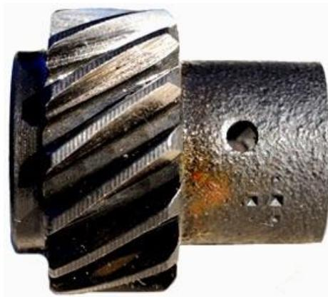
**Figure 22: Gear corrosive wear**
