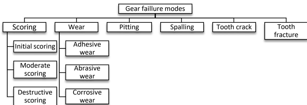
Figure 16: Gear defects classification
