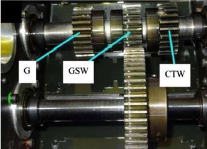
Figure 48: Single stage gear pinions location in the gearbox.
