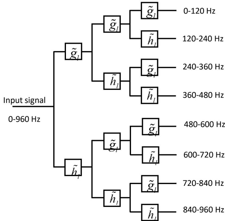
Figure 28: Three levels of the MODWPT decomposition
