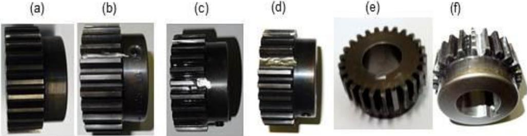
Figure 47: Six pinion states: G (a); TRC (b), CTL (c), CTW (d), MT (e) and GSW (f).
