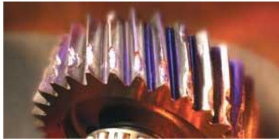
**Figure 21: Gear abrasive wear**
