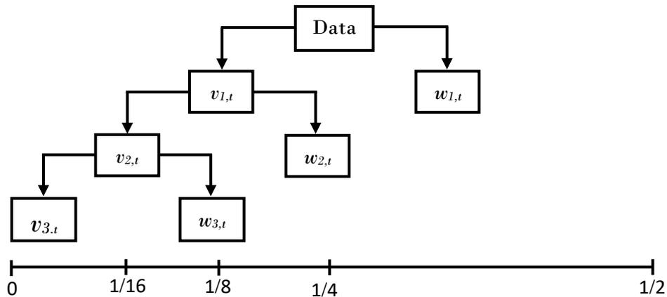
Figure 27: Decomposition process using DWT
