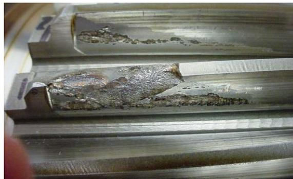
**Figure 24: Spalling defect**
