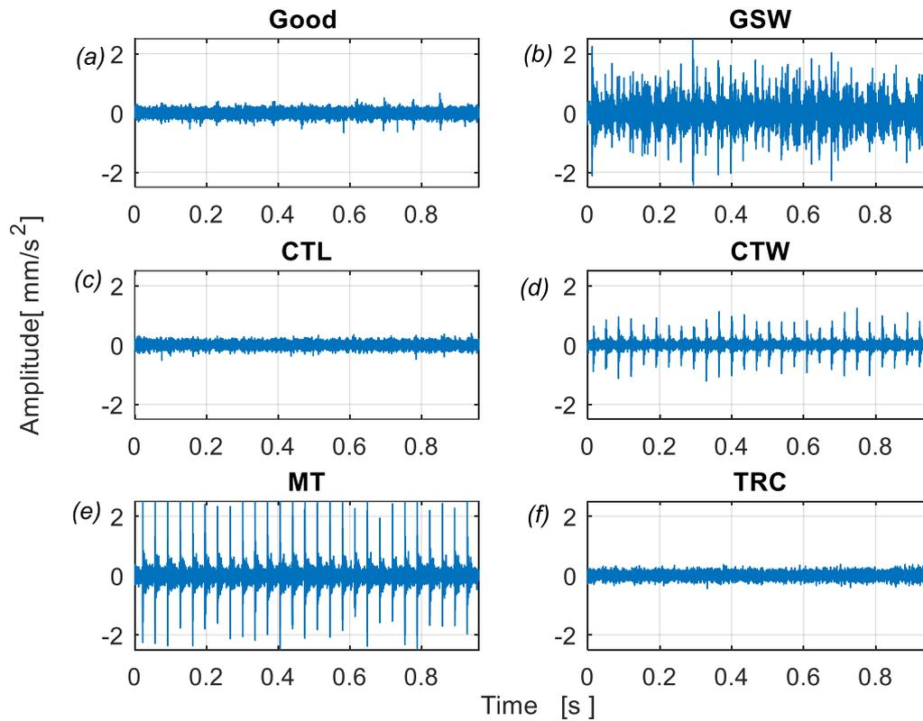
**Figure 49: Pinion vibration signals of gearbox with different faults (Speed: 900 r/min, Load: 11 Nm).**
