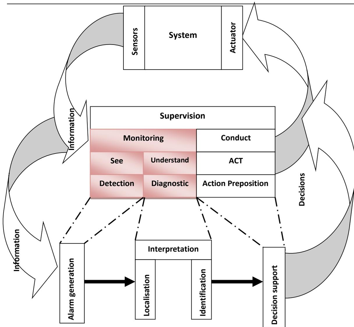
Figure 8: General process of system's supervision.
