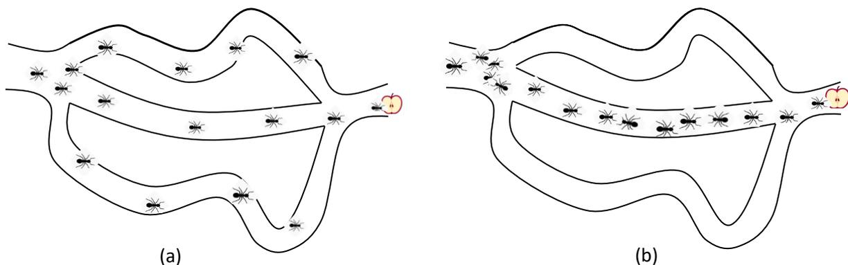
**Figure 44: Basic explanation of the ant colony algorithm.**
