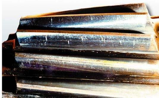
**Figure 20: Gear adhesive wear**
