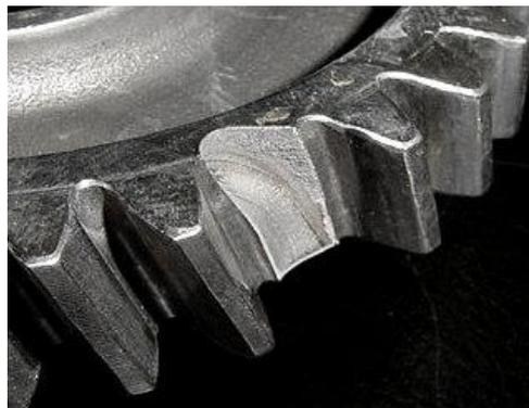
**Figure 26: Tooth fracture**
