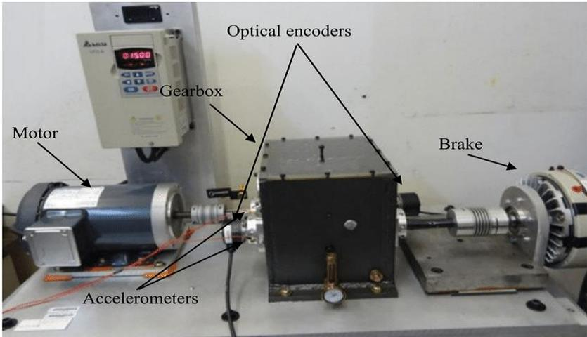
Figure 46: The gearbox test bench.
