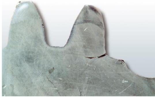
**Figure 25: Tooth crack**
