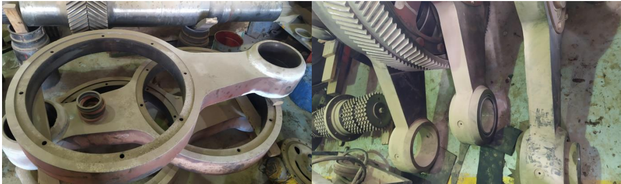
Figure 24: Bielle - manivelle
