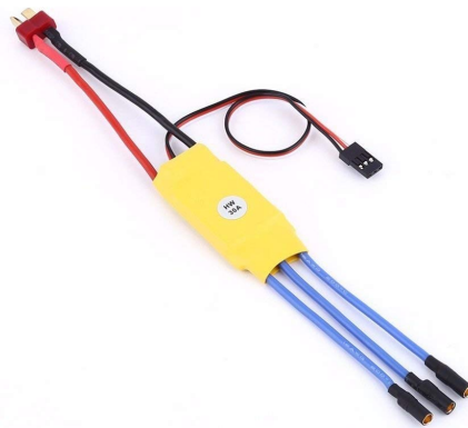
(b) 30A electronic speed controller
