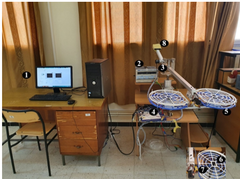
Figure 0.3. 3-DOF test bench at IGEE, (1) computer, (2) Power supply, (3) Encoder, (4) DAQ-board, (5) Motors: front on the left, (6) Motor+Propeller, (7) ESC, (8) Counterweight.
