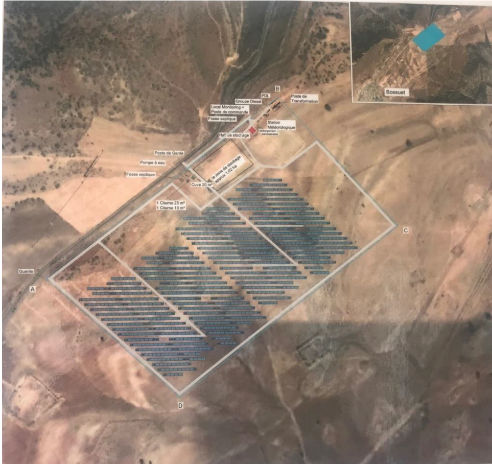
Figure 28. The general diagram of the Dhaya photovoltaic power plant in Sidi Bel Abbés[59].
