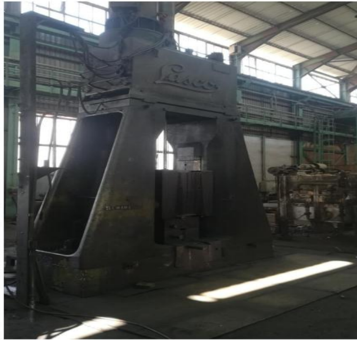
Figure II. 9: Marteau Pilon simple effet.
