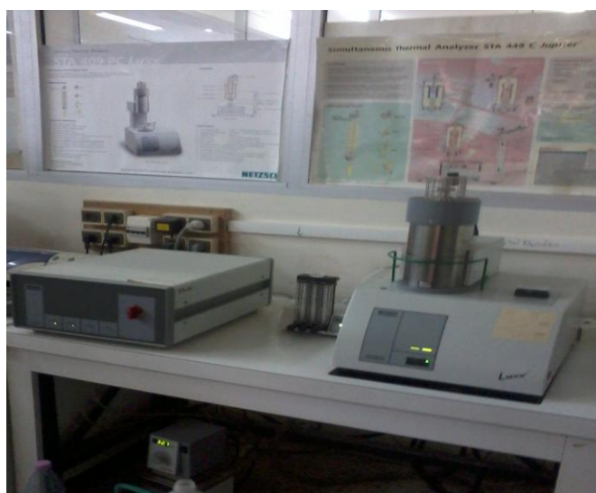
Figure 27: Appareil DSC NETZSCH STA 409 PC
