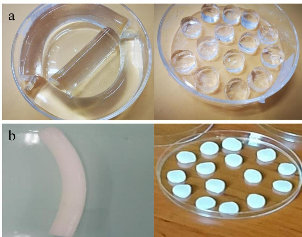
**Figure I.1.** Photographies des hydrogels (a) hydrogel de PVOH-g-poly (AA) (b) hydrogel de PVOH-g-poly (AA-co-AMPS).
