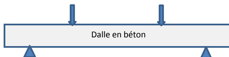
Figure IV.1: Dalle non renforcée (R)
