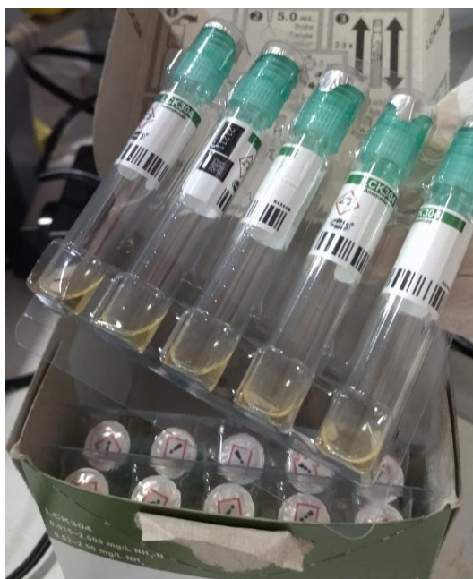
Test en cuve ammonium 0.015-2 MG/L LCK304
